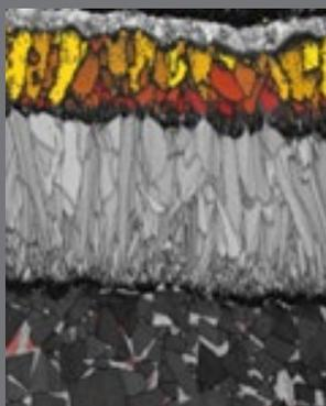
In conventional CVD alumina coatings, the crystal orientation is random.
