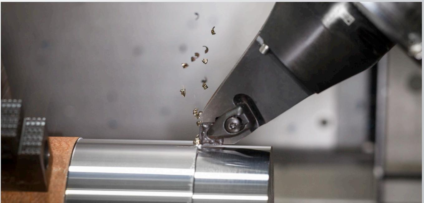
So, how is this possible? Well, the insert substrate and coating of GC4325 are highly capable of maintaining the insert edge line at higher temperatures, which translates into the potential for higher cutting speeds with added security through more predictable, longer tool life. As a result, an average productivity increase of 30 per cent over other existing technologies is now readily available.
