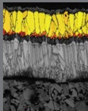
With Inveio™, every crystal in the alumina coating is lined up in the same direction, towards the top surface.
